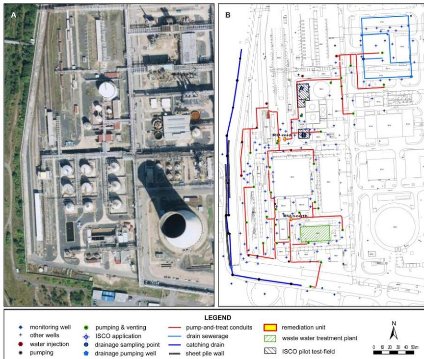
Figure 2. Aerial photograph of the petrochemical facility area impacted with the contaminant plume (www.mapy.cz); B, remediation project design.
